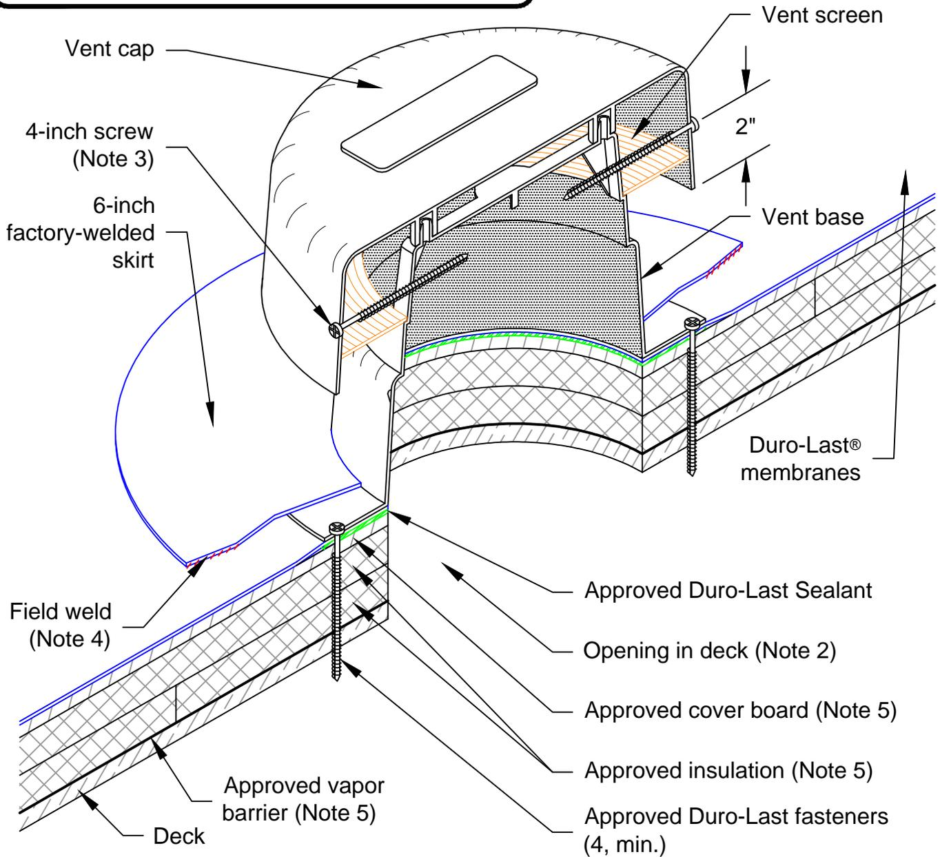
**Note 1: Only to be used for passive venting of unconditioned attic space.**
