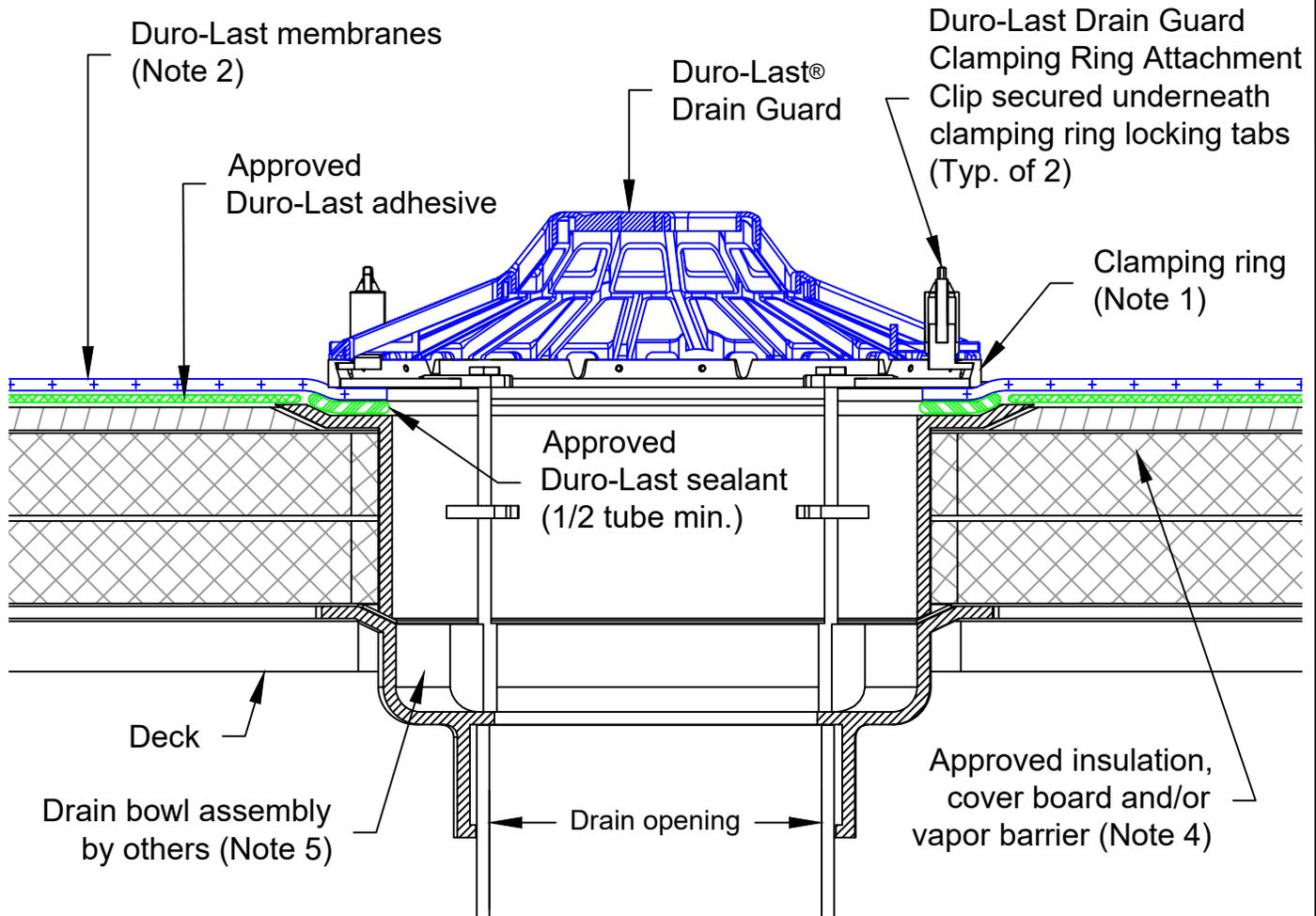
Note 1: Compatible clamping rings: Watts B2-FLG, Zurn 56588, Zurn 29480, Wade W-3000-I-FRG, JR Smith 3260 and JR Smith 35400.
