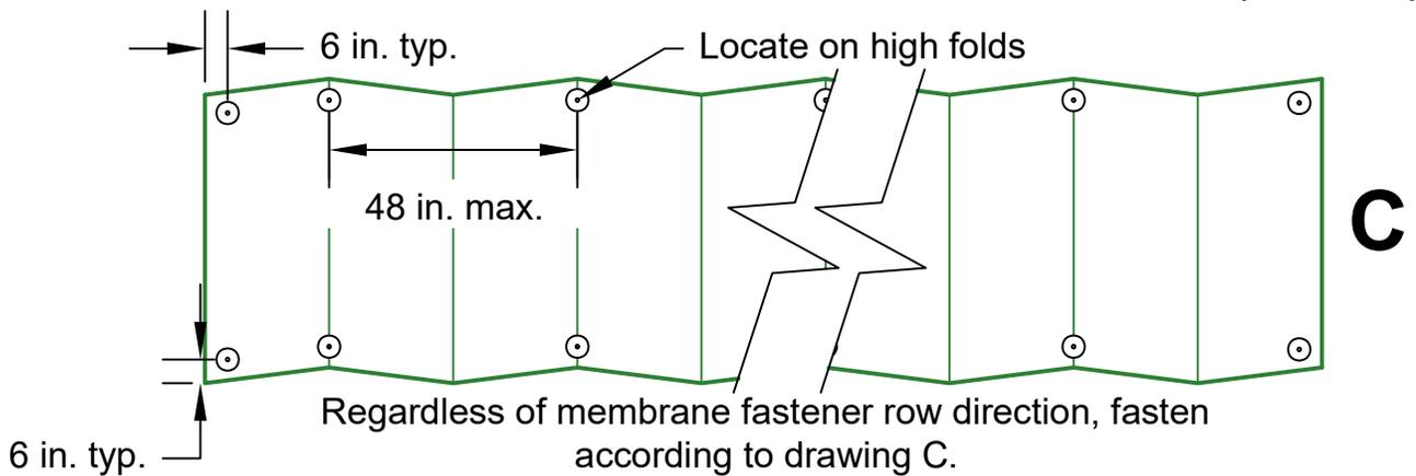
Note: Do **not** damage the fan fold board or facer by overdriving fasteners.
