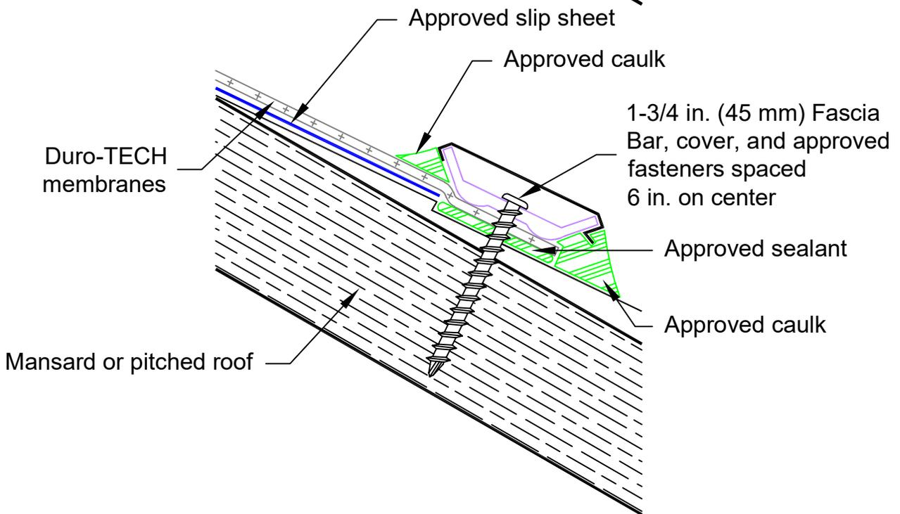
Note 1: The mansard slope must be a minimum of 3 in./ft (1:4).
