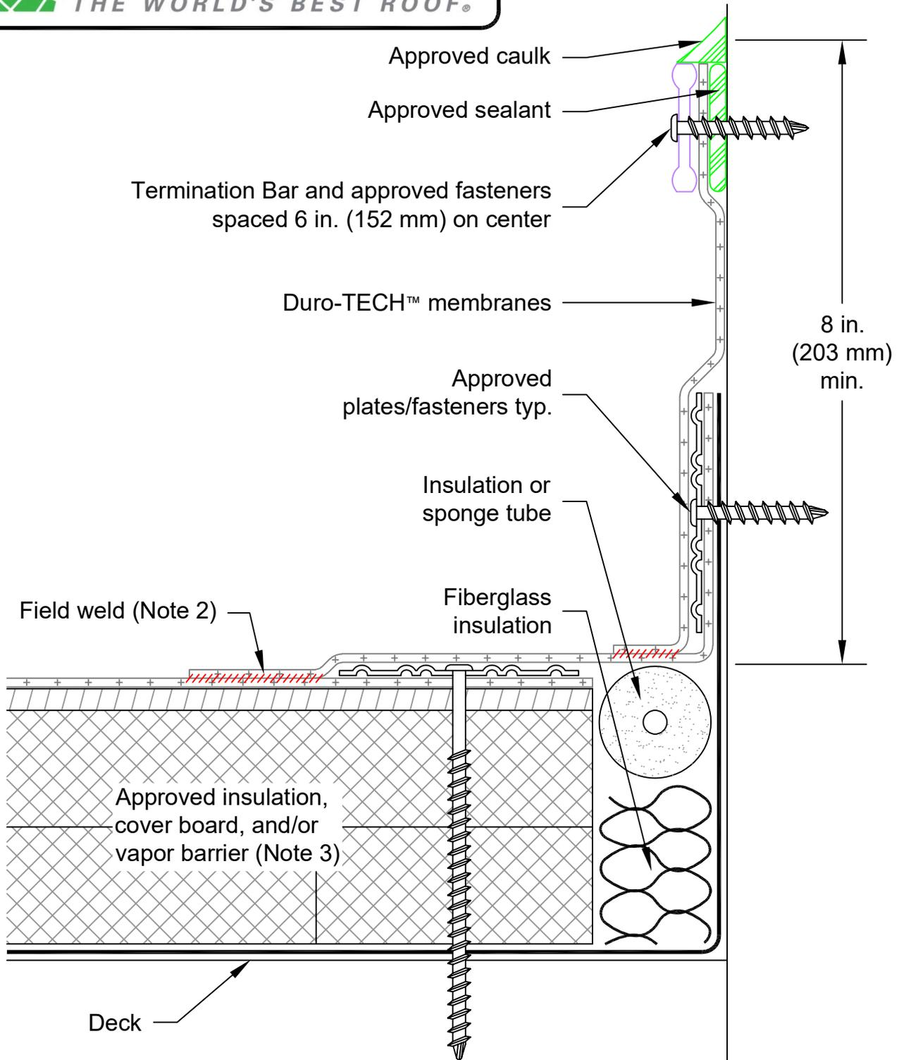
Note 1: Membrane parallel to the expansion joint must be mechanically fastened with the same fastening pattern used on the membrane in the field area.
