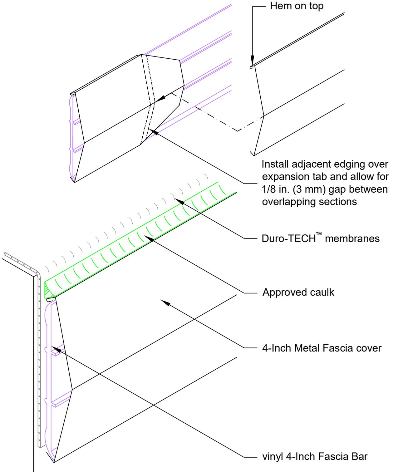
Note 1: This detail may also be used on parapet walls.
