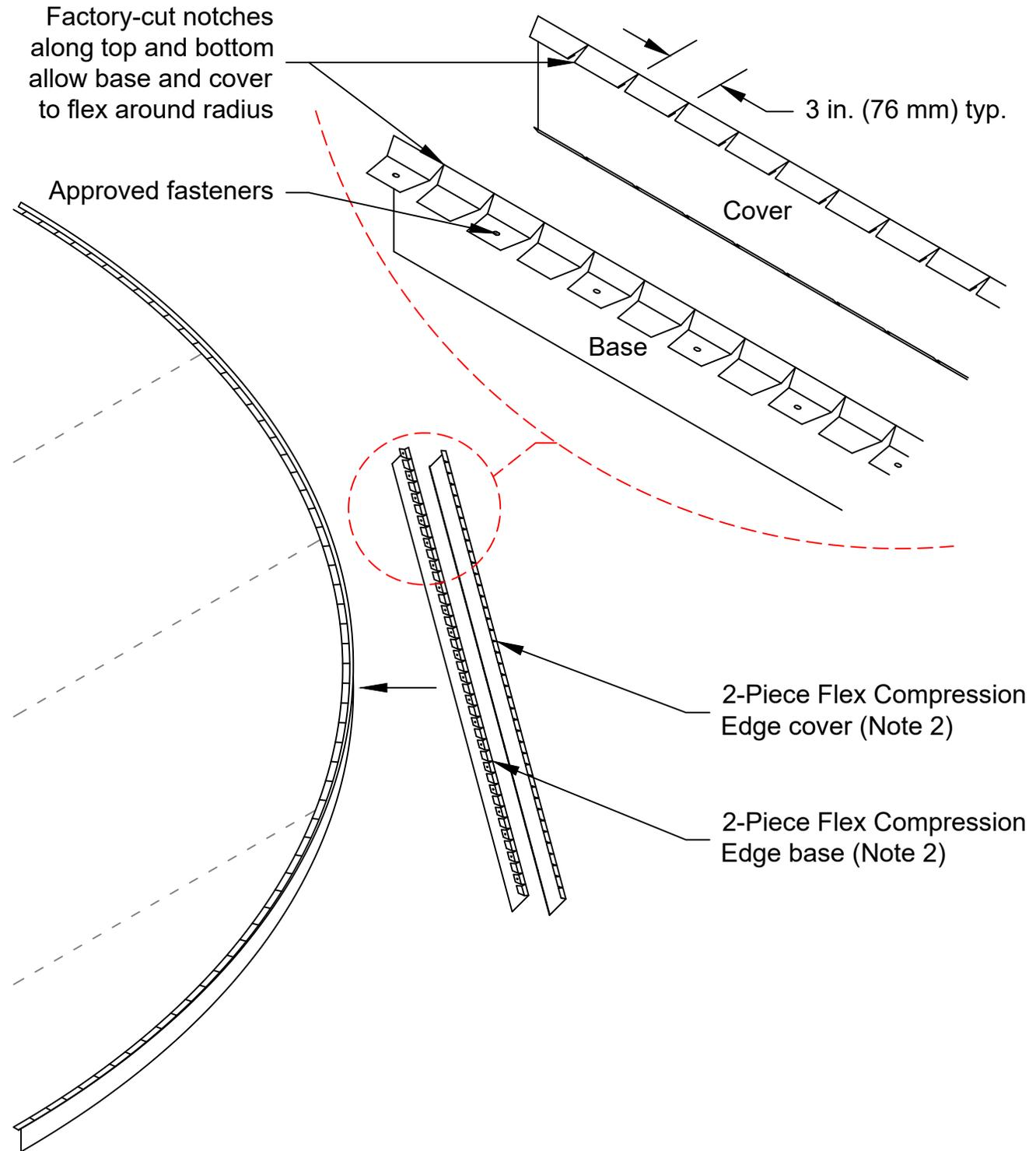
Note 1: This detail may also be used on parapet walls.
