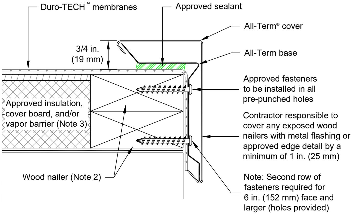
Note 1: Overlap each 10 ft (3 m) length of base by 1 in. (25 mm). Overlap the covers by 1-1/2 in. (40 mm) utilizing the pre-notched end on 10 ft (3 m) lengths.
