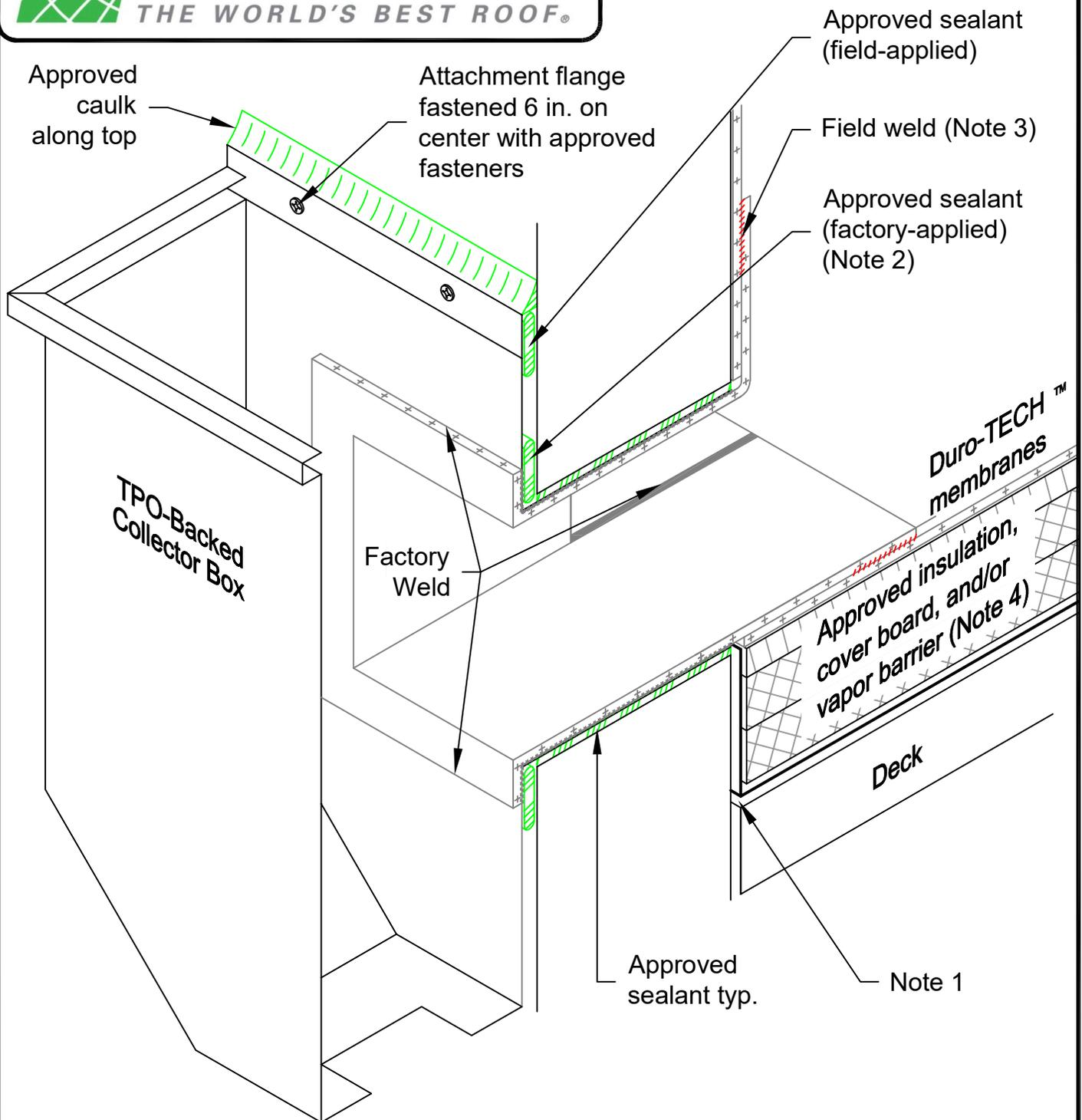
Note 1: Precaution must be taken to ensure that all deck-to-wall transitions are sealed.
