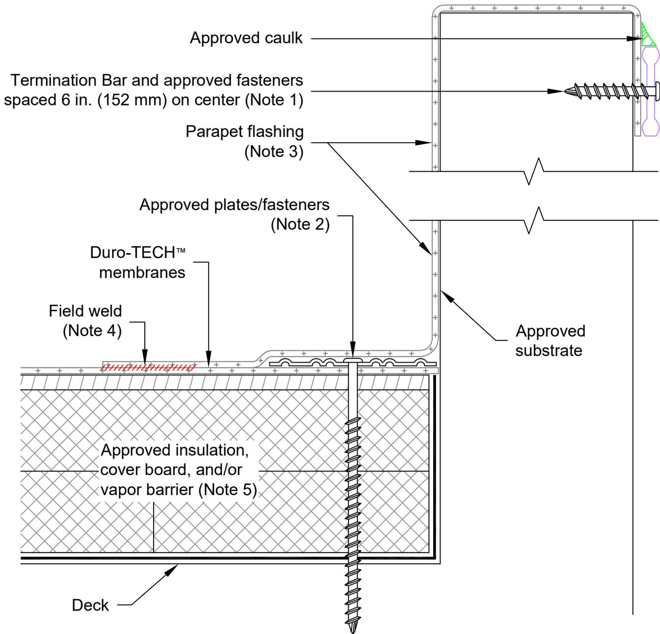
Note 1: Approved edge details may be used in place of Termination Bar.
