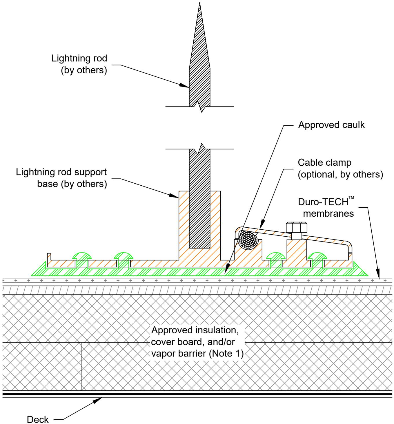
Note 1: Refer to specifications for vapor barrier, insulation, and cover board requirements.
