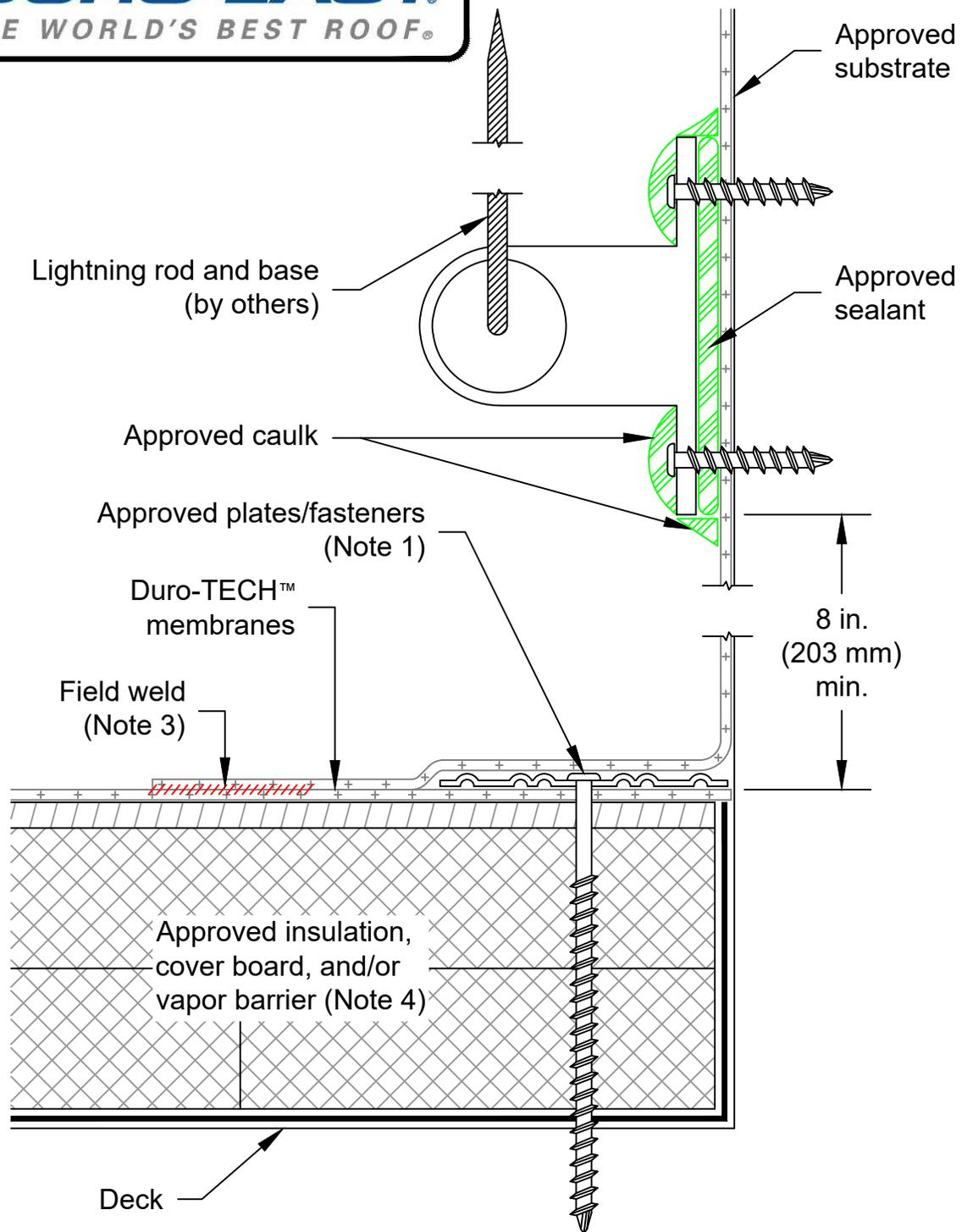
Note 1: Membrane fastening at deck-to-wall transitions and walls must be same as per respective zones that area is located within (field, perimeter, corner).
