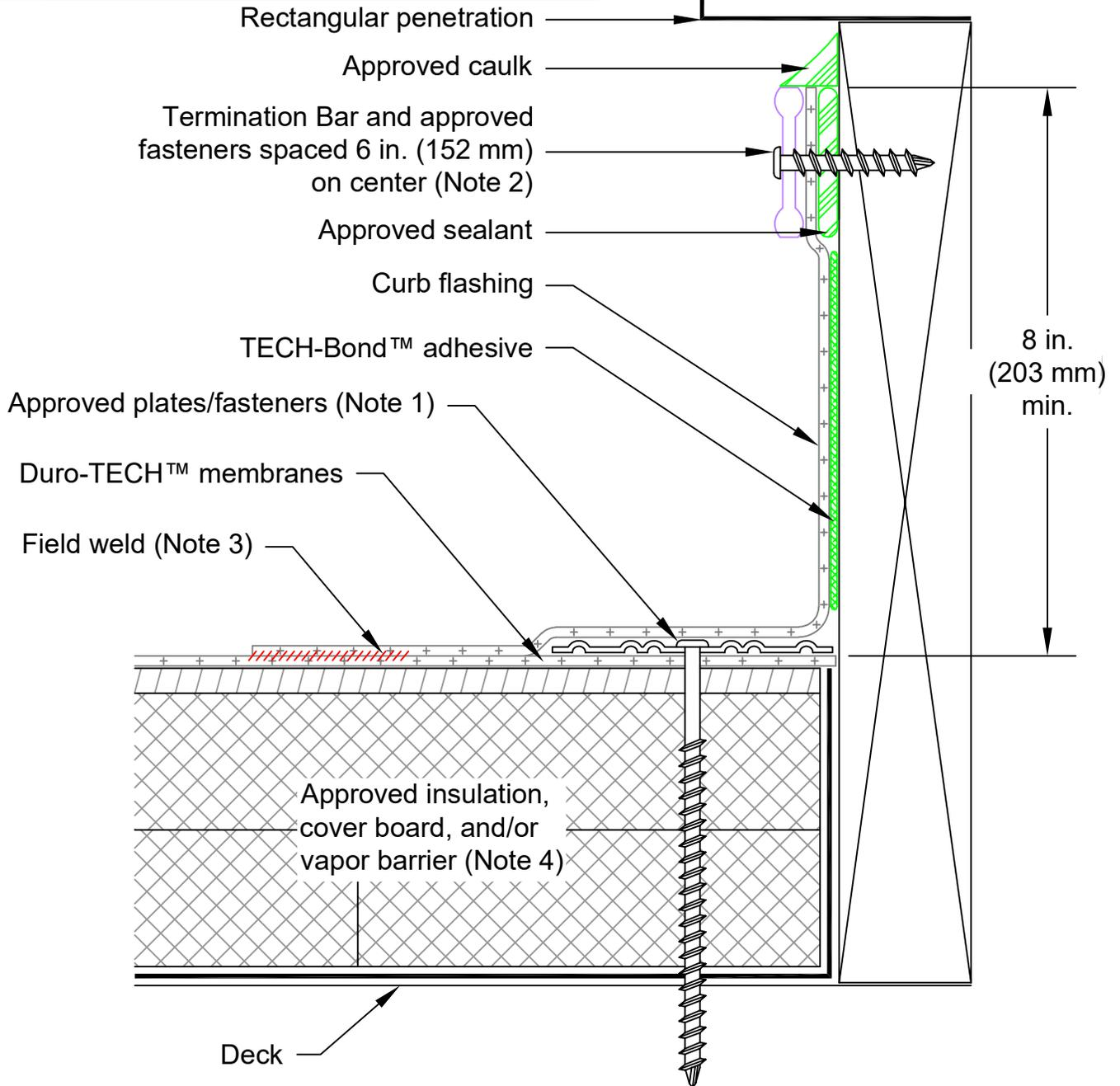
Note 1: Deck membrane must be fastened around perimeter of roof penetration as per respective zone the roof access hatch is located within (field, perimeter, corner).
