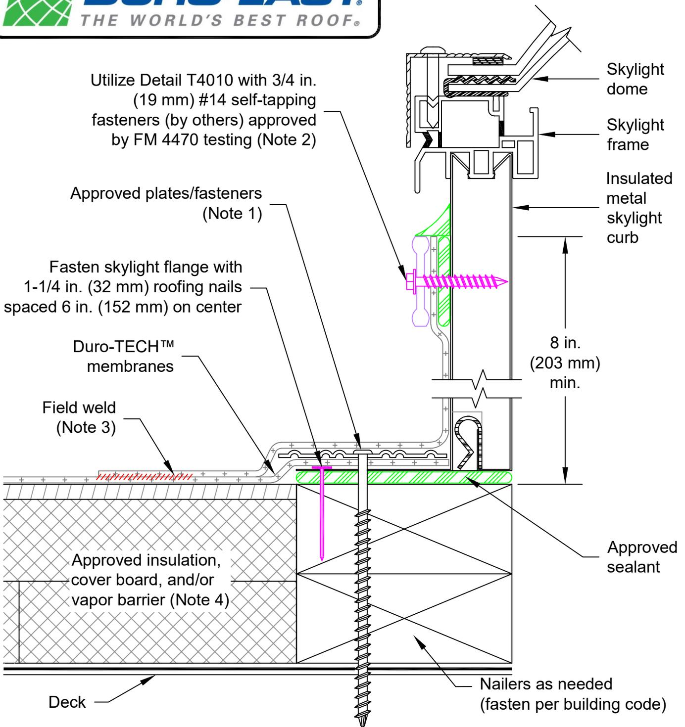
Note 1: Deck membrane must be fastened around perimeter of roof penetration as per respective zone the skylight is located within (field, perimeter, corner).
