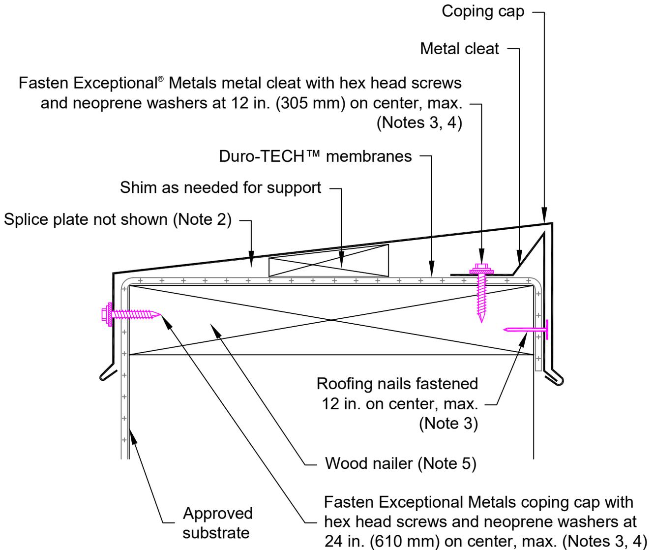
Note 1: All coping cap joints must utilize a 6 in. (152 mm) concealed splice plate.
