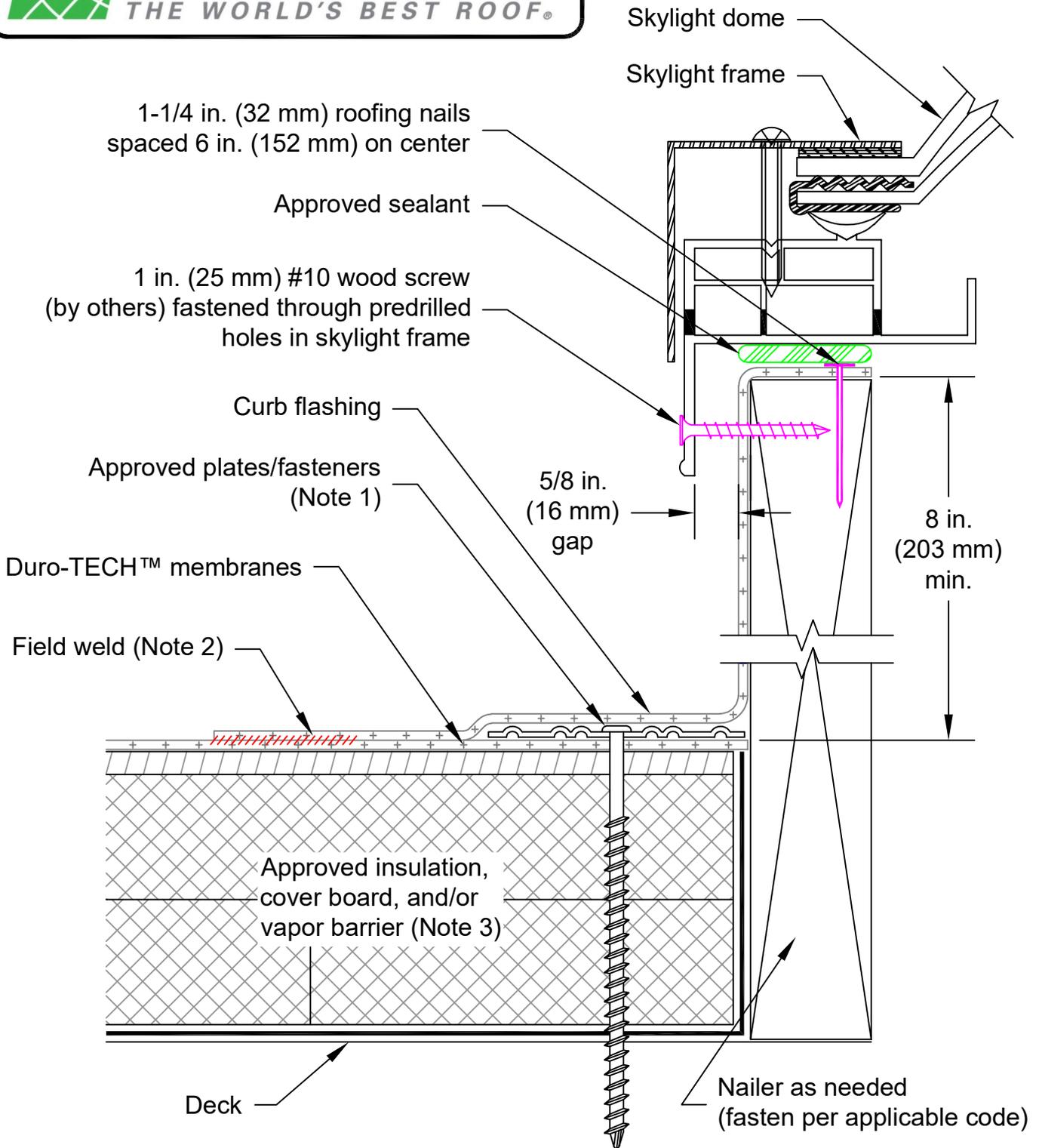
Note 1: Deck membrane must be fastened around perimeter of roof penetration as per respective zone the skylight is located within (field, perimeter, corner).
