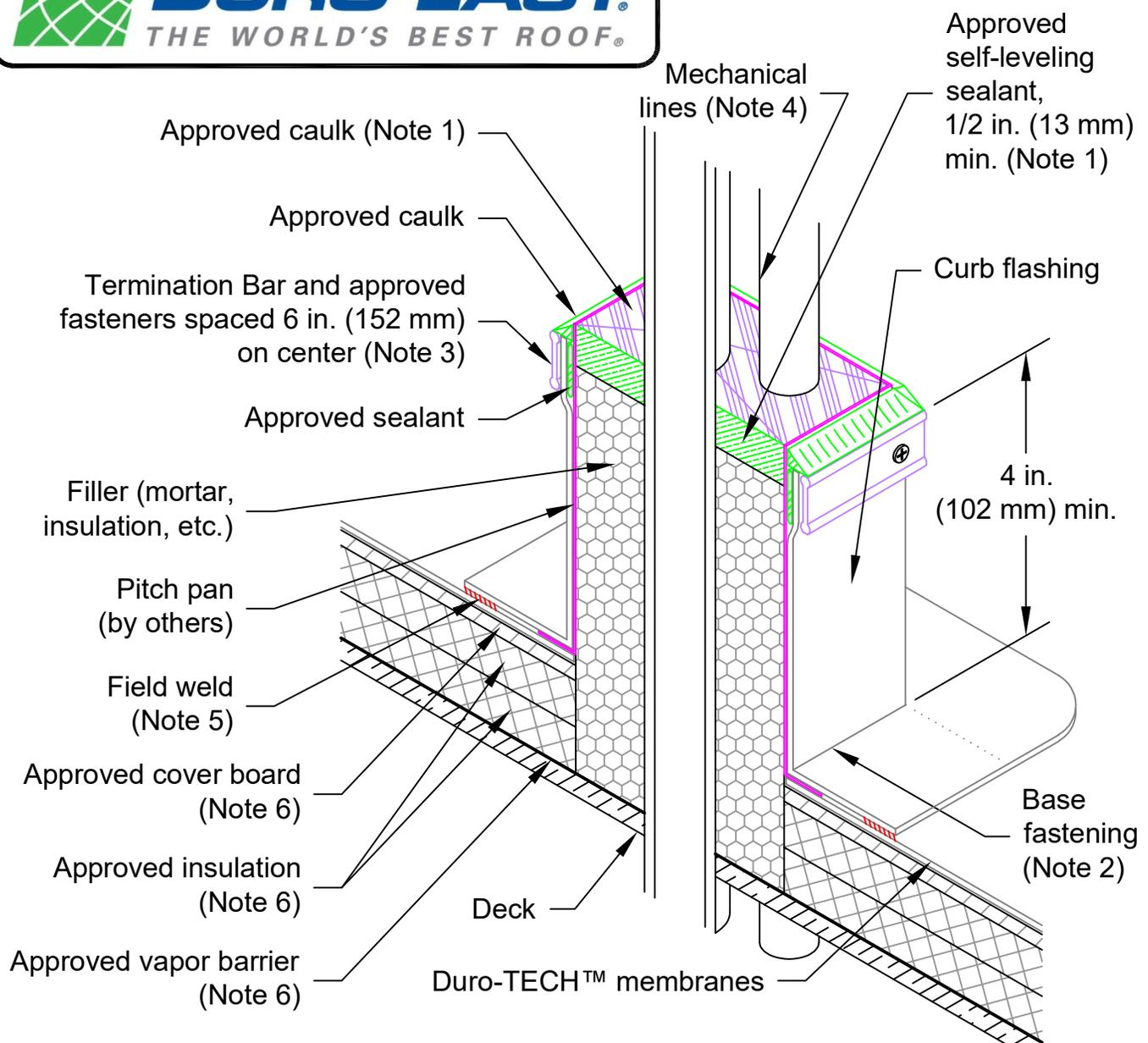
Note 1: Water must not be allowed to pond within pitch pan. Ensure that approved self-leveling sealant is level with top of curb. Cover with approved caulk to slope to outside of pitch pan.
