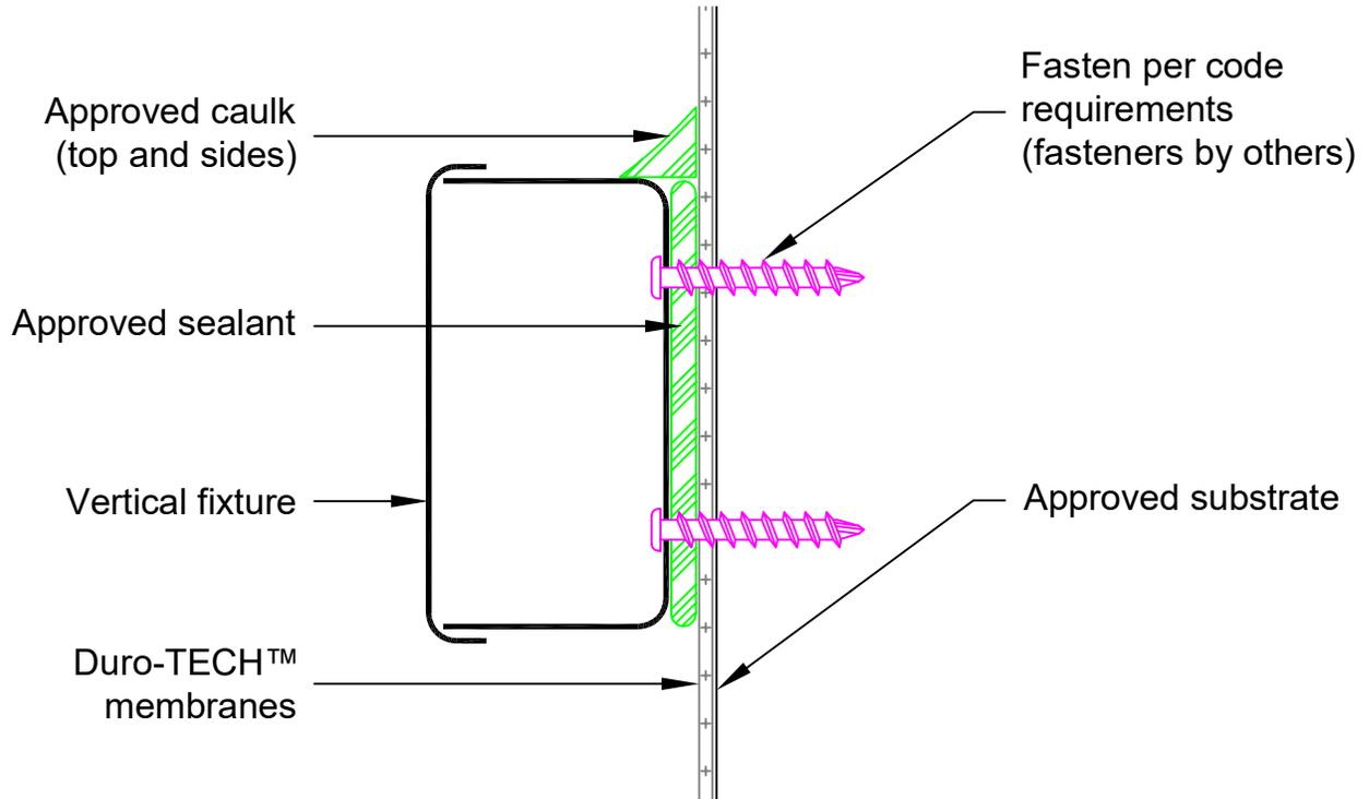
Note: Bottom of vertical fixture shall be a minimum of 8 in. (203 mm) above the finished roof deck.
