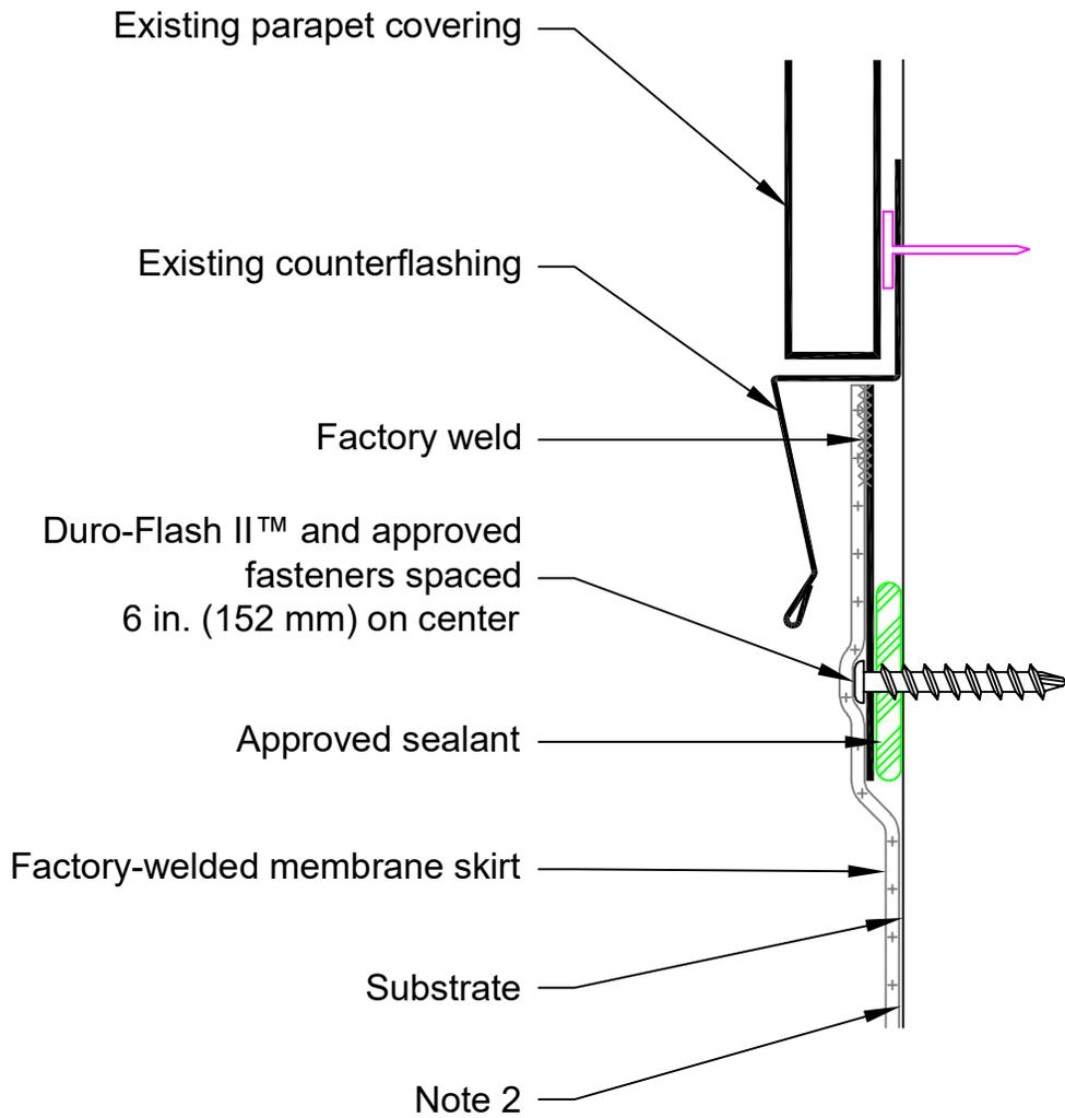
Note 1: Minimum termination height for parapet flashing is 8 in. (203 mm) above finished deck. Refer to Detail T6020.
