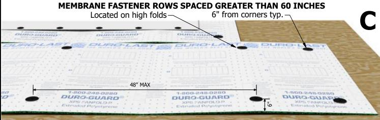
Regardless of membrane fastener row direction, fasten according to drawing C.
