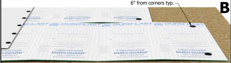
If membrane fastener row run perpendicular to 50-ft board dimension, fasten according to drawing B.
