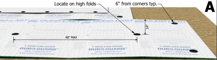
If membrane fastener rows run parallel to 50-ft board dimension, fasten according to drawing A.
