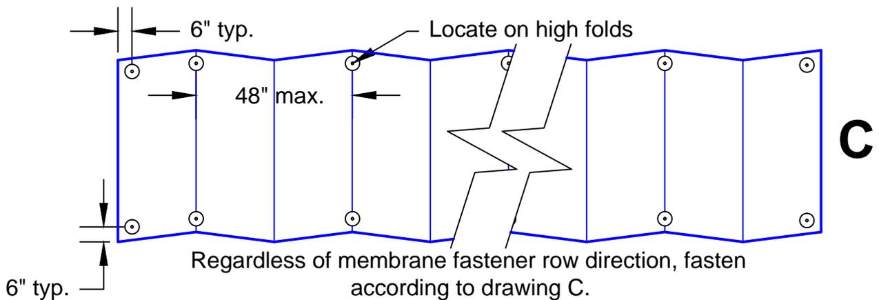
Note: Do not overdrive the fasteners. Overdriven fasteners might crush the fan fold board or tear the facer.
