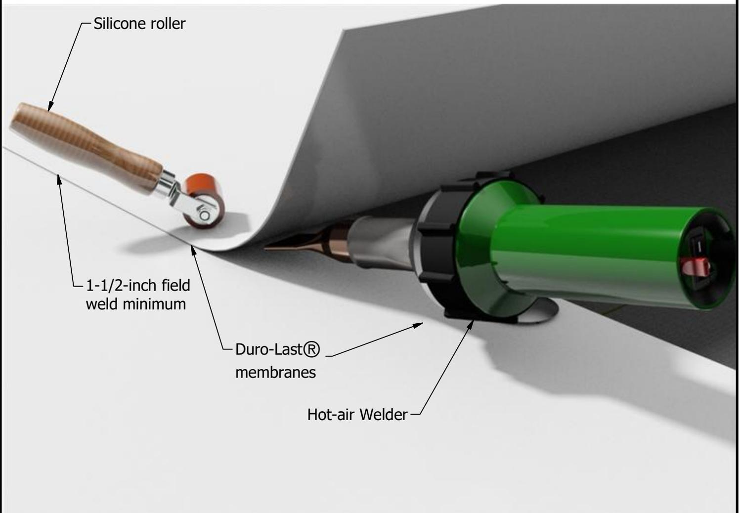
Note: After any field seam is completed, it must be probed to ensure that a secure weld has been made.
