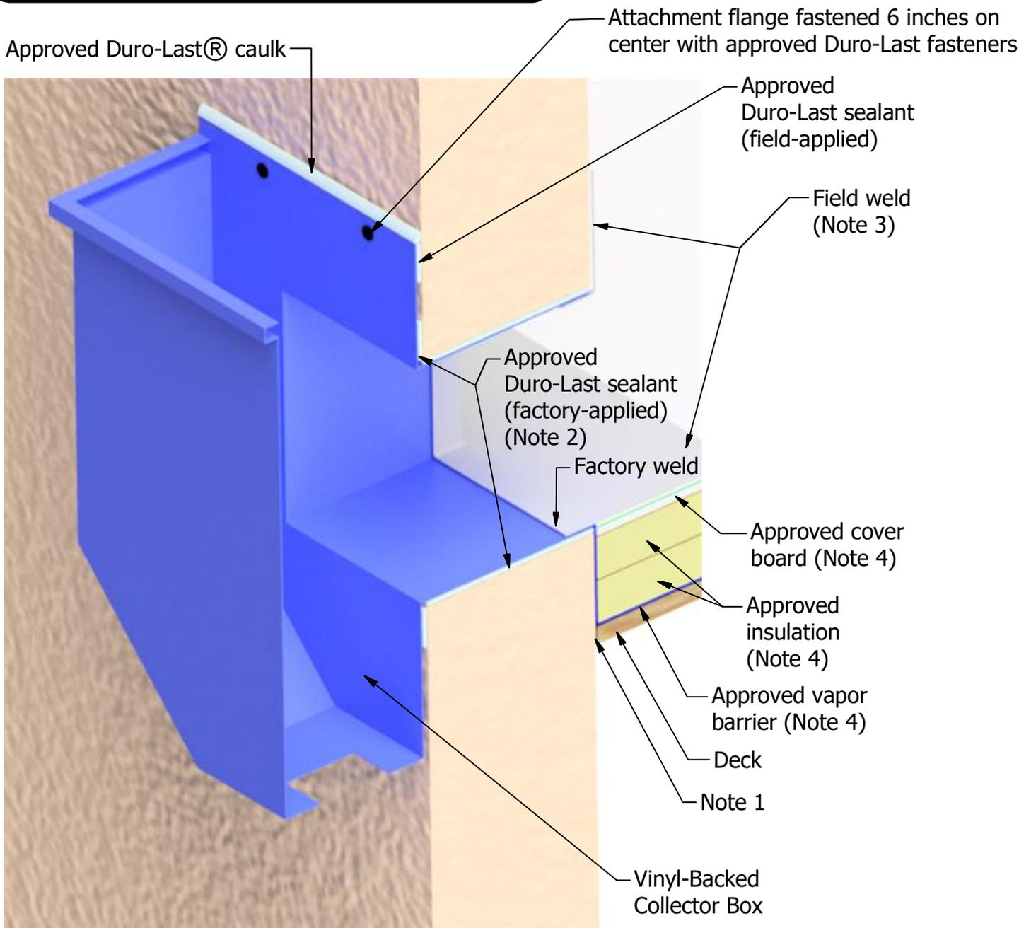
Note 1: Precaution must be taken to ensure that all wall-to-deck transitions are sealed.
