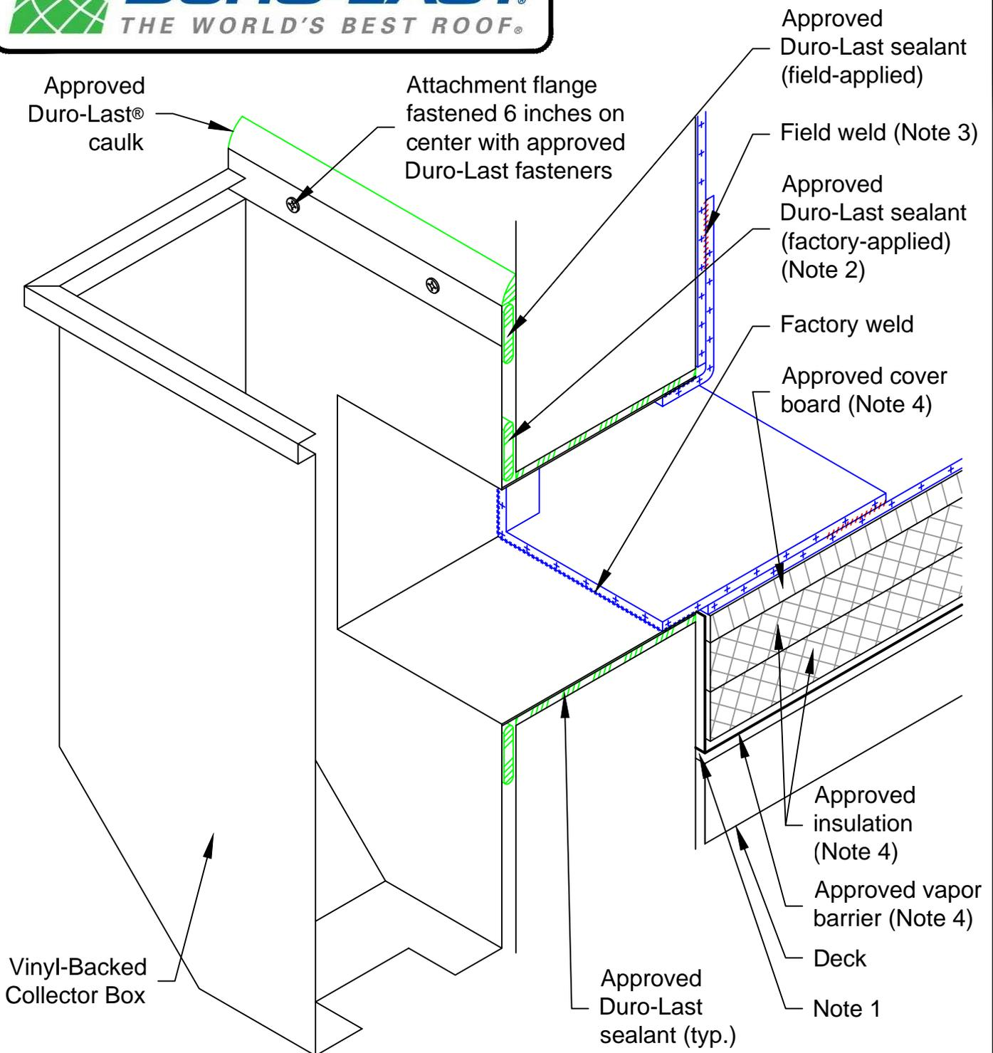
Note 1: Precaution must be taken to ensure that all wall-to-deck transitions are sealed.
