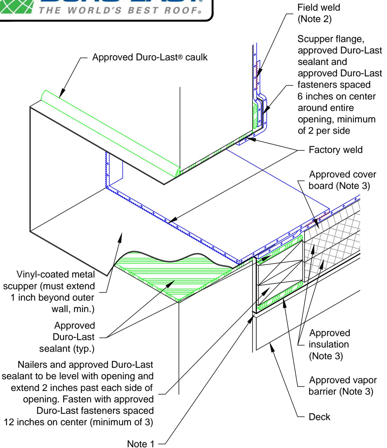
Note 1: Precaution must be taken to ensure that all wall-to-deck transitions are sealed.
