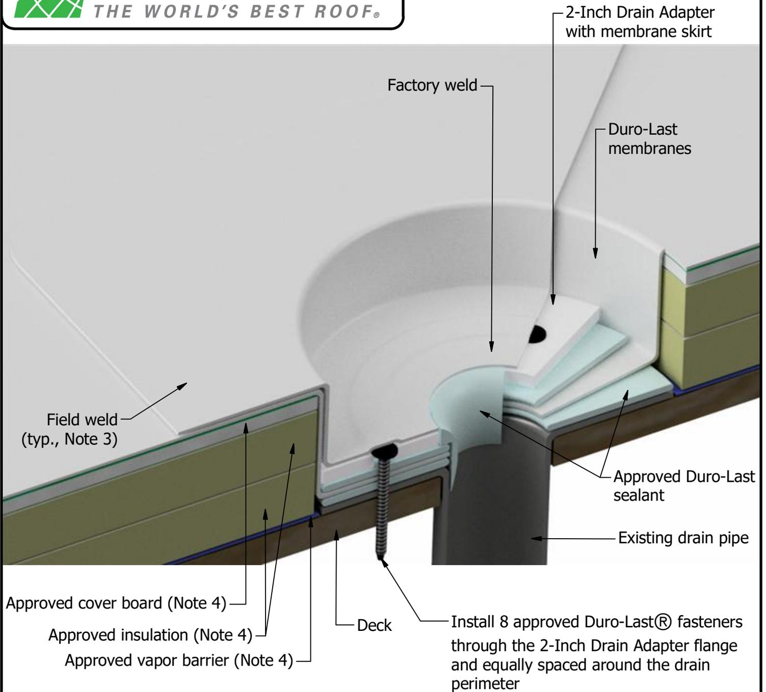
Note 1: This detail cannot be used on drains larger than 2 inches in diameter.
