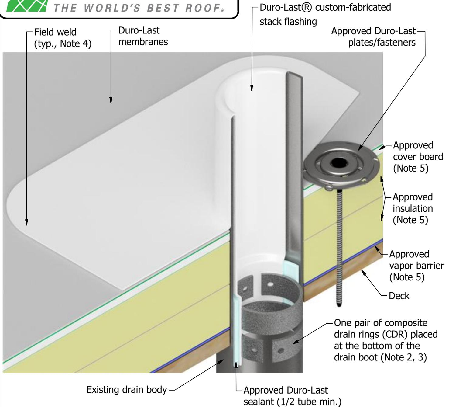
Note 1: Membrane must be fastened around the perimeter of the drain with the same fastening pattern as the field membrane, no less than one fastener per drain.
