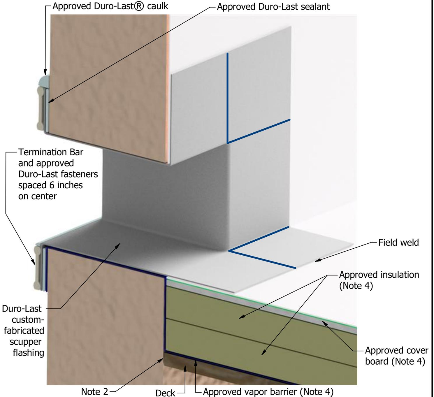
Note 1: Deck and wall membrane shall be fastened around the perimeter of the scupper opening as per the respective zone the scupper is located within (field, perimeter, corner), no less than one fastener per side.
