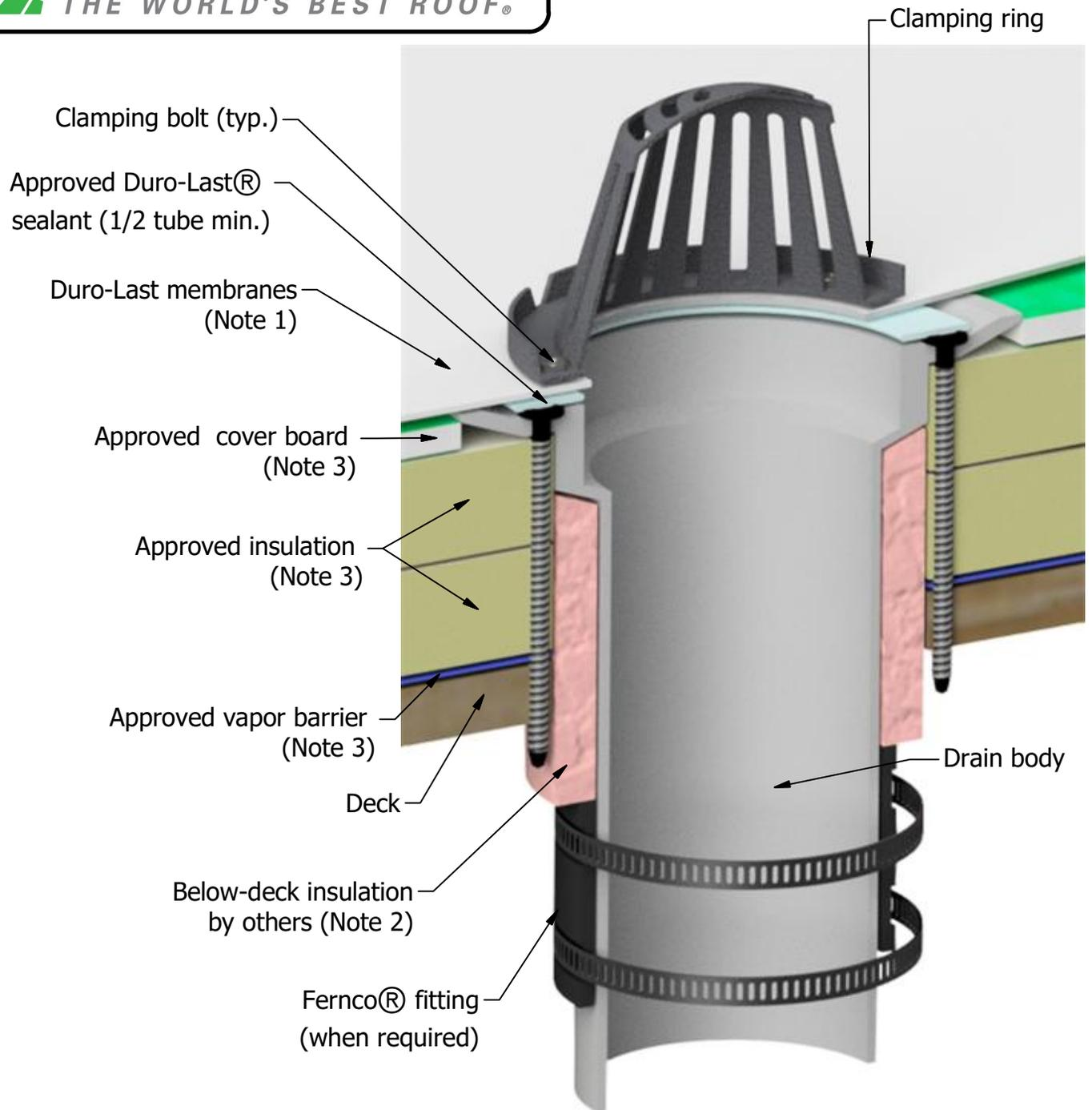
Note 1: Duro-Last membrane must extend beyond the inside of the clamping ring. The hole in the membrane must be larger than the drain pipe diameter.
