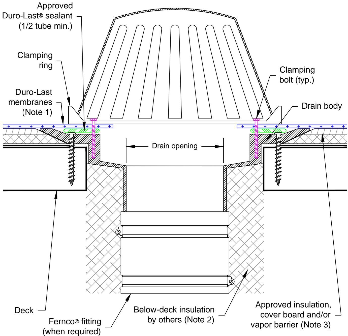
Note 1: Duro-Last membrane must extend beyond the inside of the clamping ring. The hole in the membrane must be larger than the drain pipe diameter.
