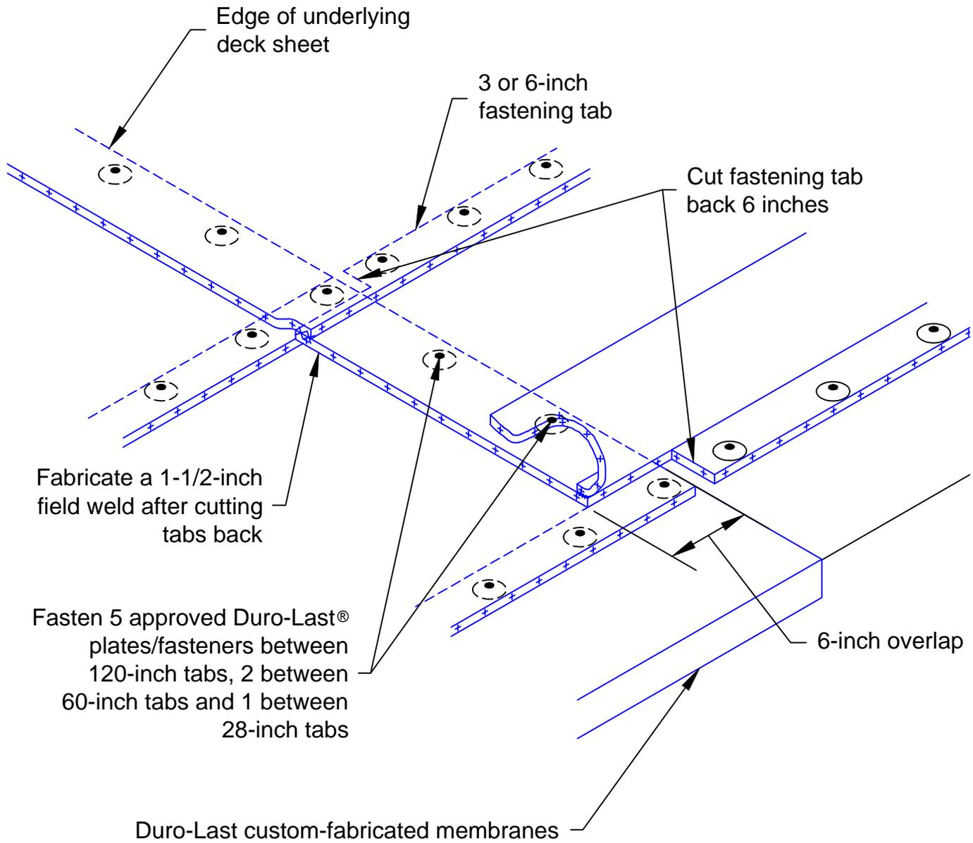
Note 1: Overlapping 6 inches and cutting back fastening tabs allows adequate space for fastening and field seaming. When cutting back the fastening tab, be careful not to cut the top layer of membrane.
