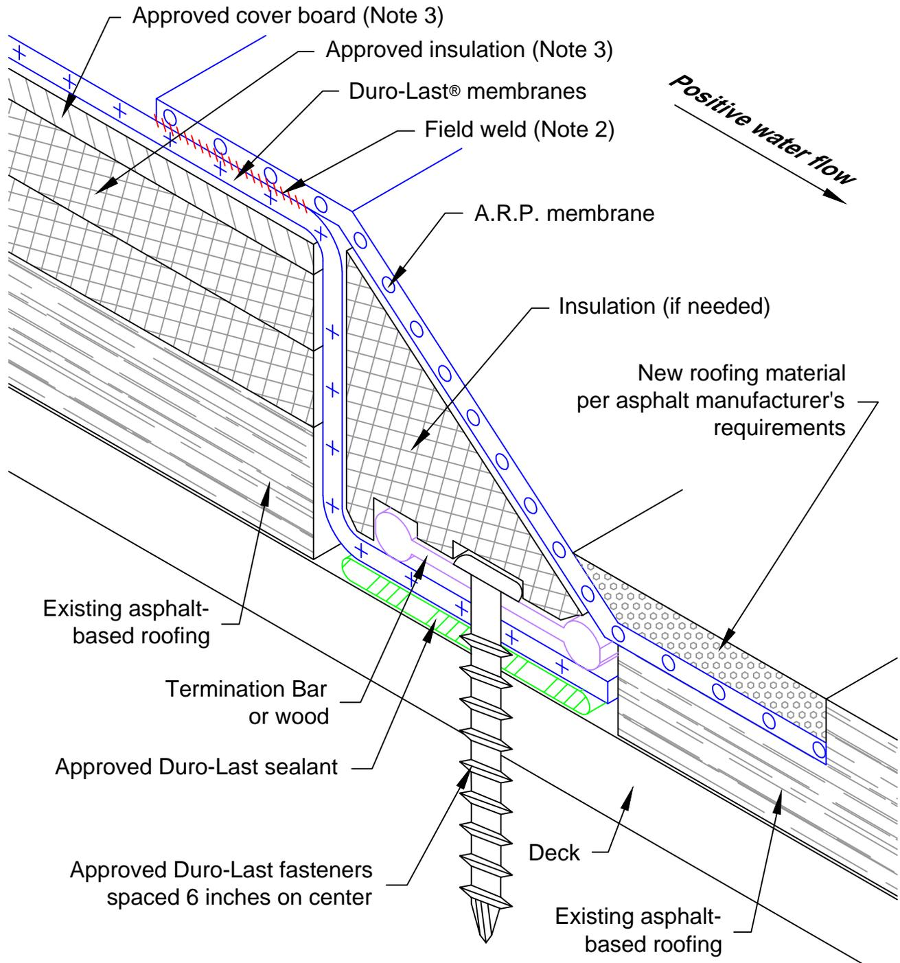
Note 1: Tie-in detail for all flat surfaces. The use of Detail Drawing 1070 will be required in conjunction with Detail Drawing 1080 when tie-in is across metal flutes.
