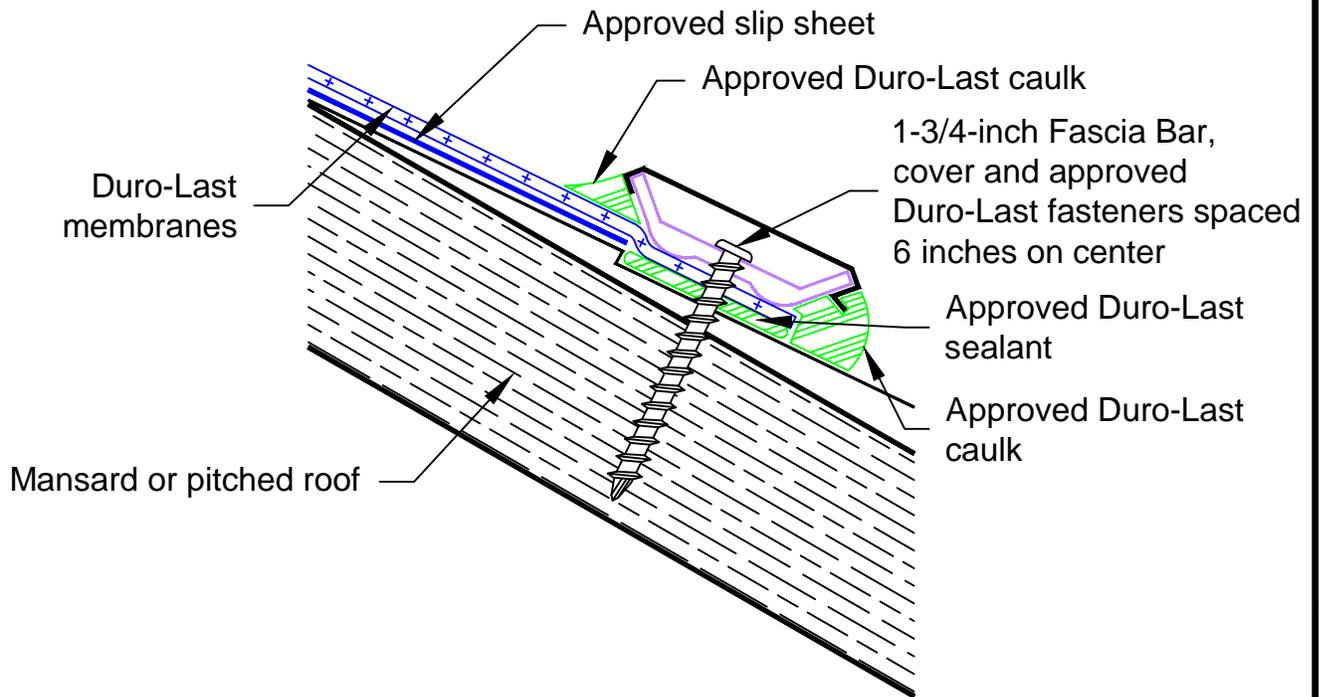
Note 1: The mansard slope must be a minimum of 3 inches vertically for every 12 inches horizontally.
