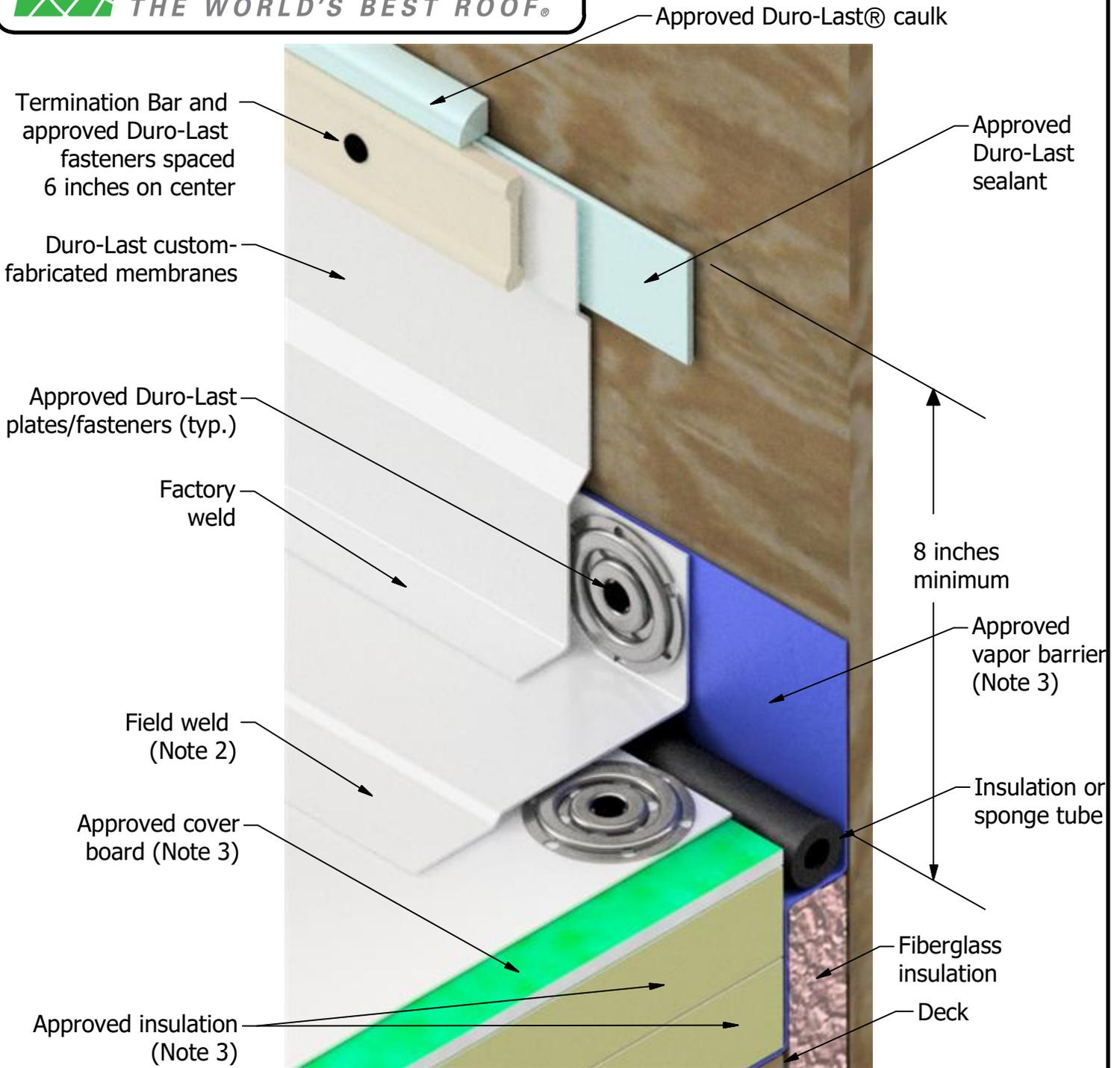
Note 1: Tabs that are parallel to the expansion joint must be mechanically fastened with the same fastening pattern used on the membrane in the field area.
