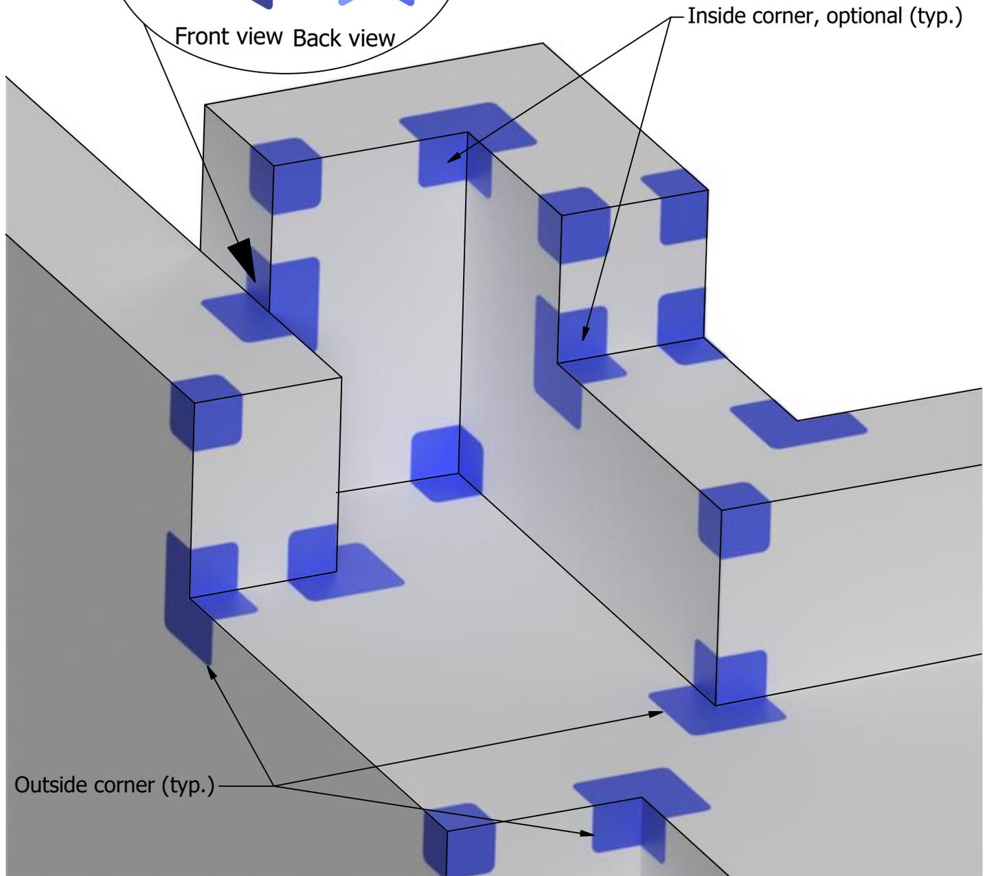
Note: Ensure that the correct side of the membrane is facing out.
