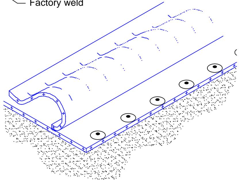
Note: On mechanically fastened systems, the fastening plates must be installed with the edge of the plate on the outside edge of the fastening tab, as illustrated above.
