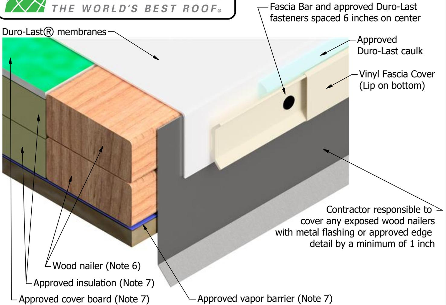
Note 1: This detail may also be used on parapet walls.
