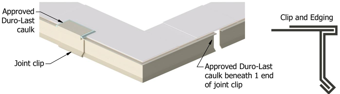
Note 1: The use of this detail is not allowed on adhered applications.
