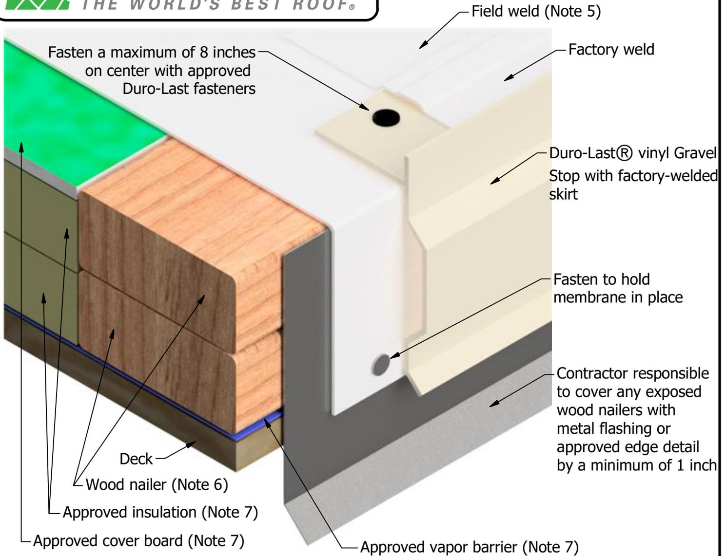
**Note 1: The use of this detail is not allowed on adhered applications.**
