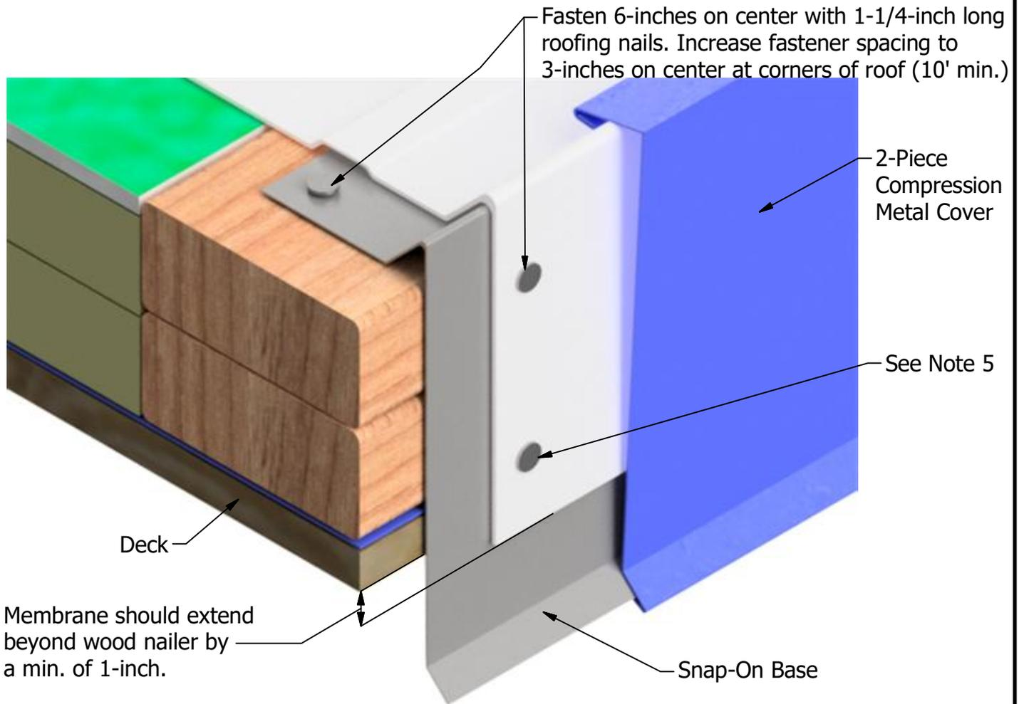
Note 1: **The use of this detail is not allowed on fully adhered installations.**
