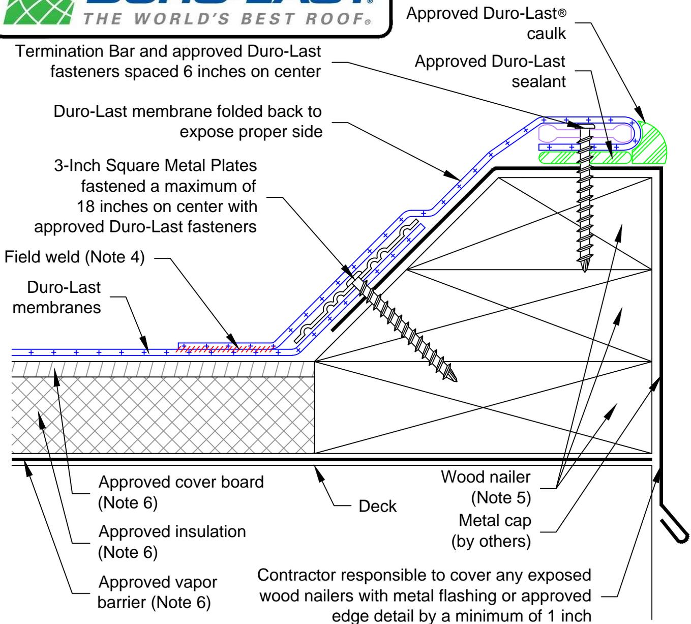
**Note 1: The use of this detail is not allowed on adhered applications.**
