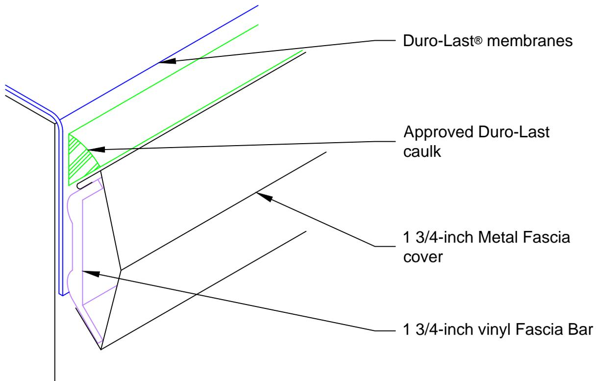
Note 1: This detail may also be used on parapet walls.
