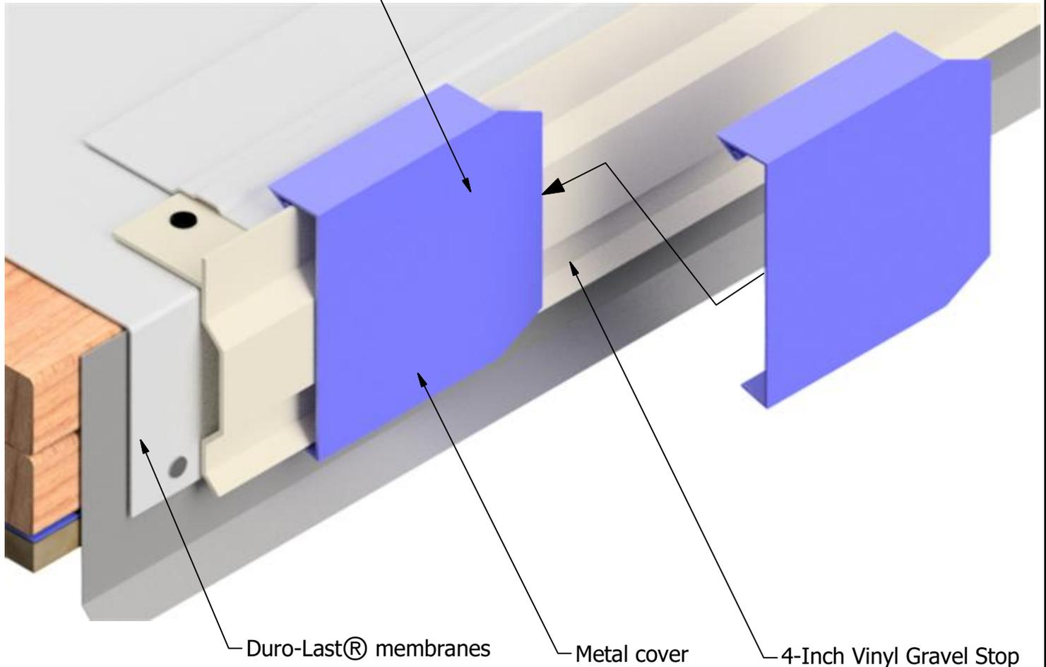
Note 1: The use of this detail is not allowed on adhered applications.
