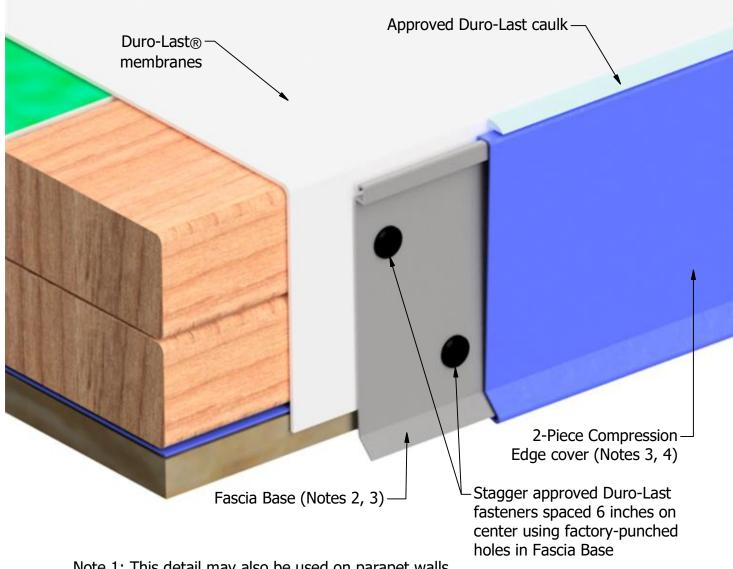
Note 1: This detail may also be used on parapet walls.
