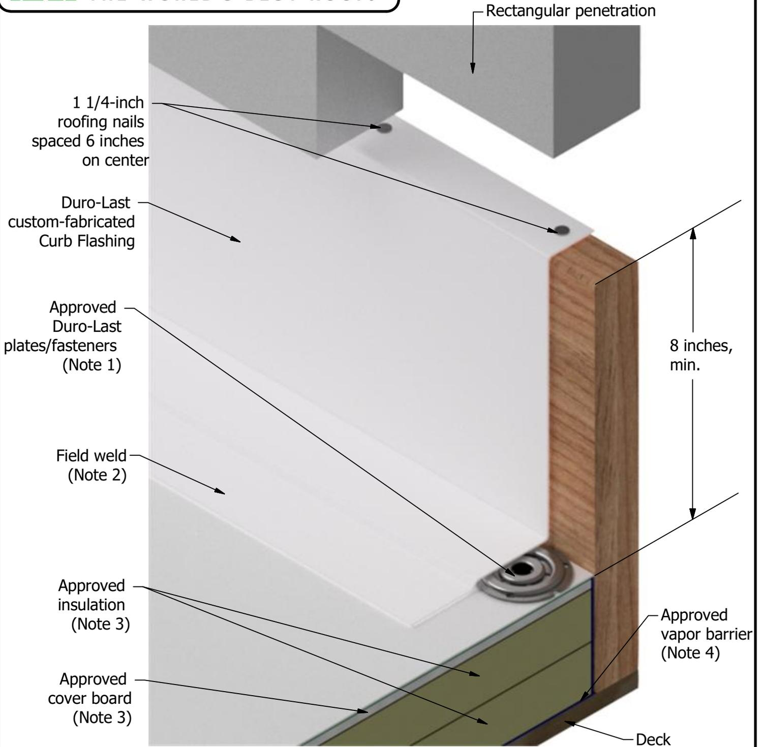
Note 1: Deck membrane shall be fastened around perimeter of roof penetration as per respective zone the roof access hatch is located within (field, perimeter, corner).
