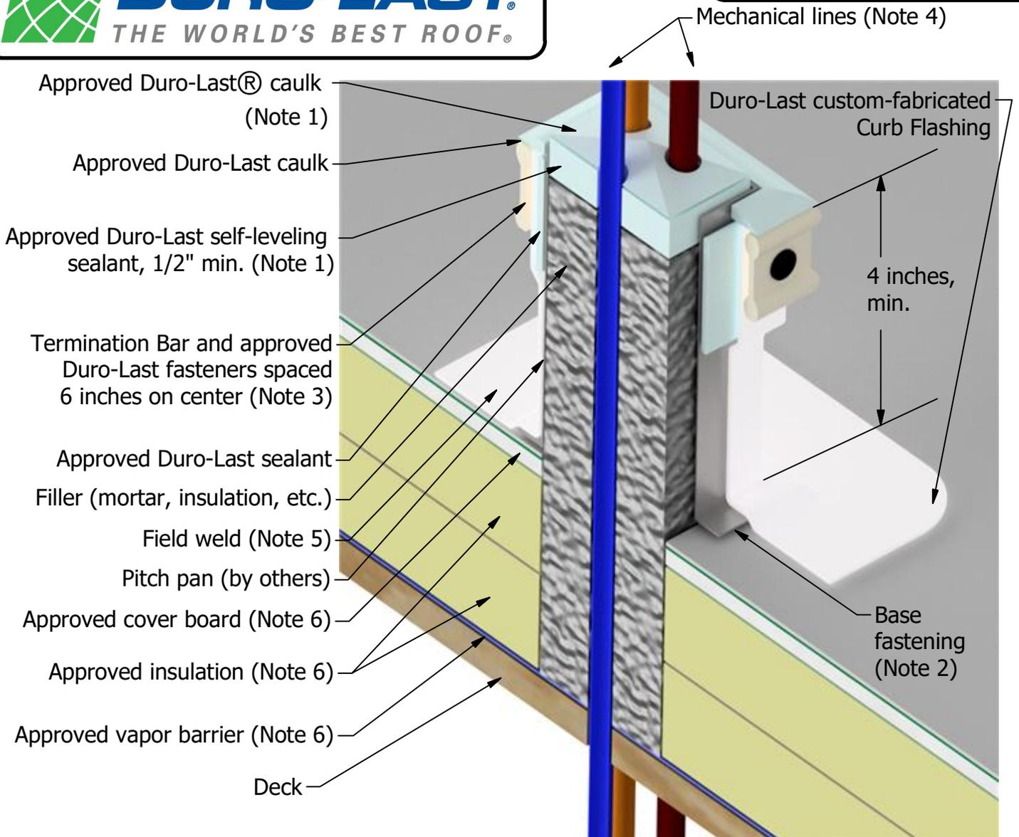
Note 1: Water must not be allowed to pond within pitch pan. Ensure that approved Duro-Last self-leveling sealant is level with top of curb. Cover with approved Duro-Last caulk to slope to outside of pitch pan.
