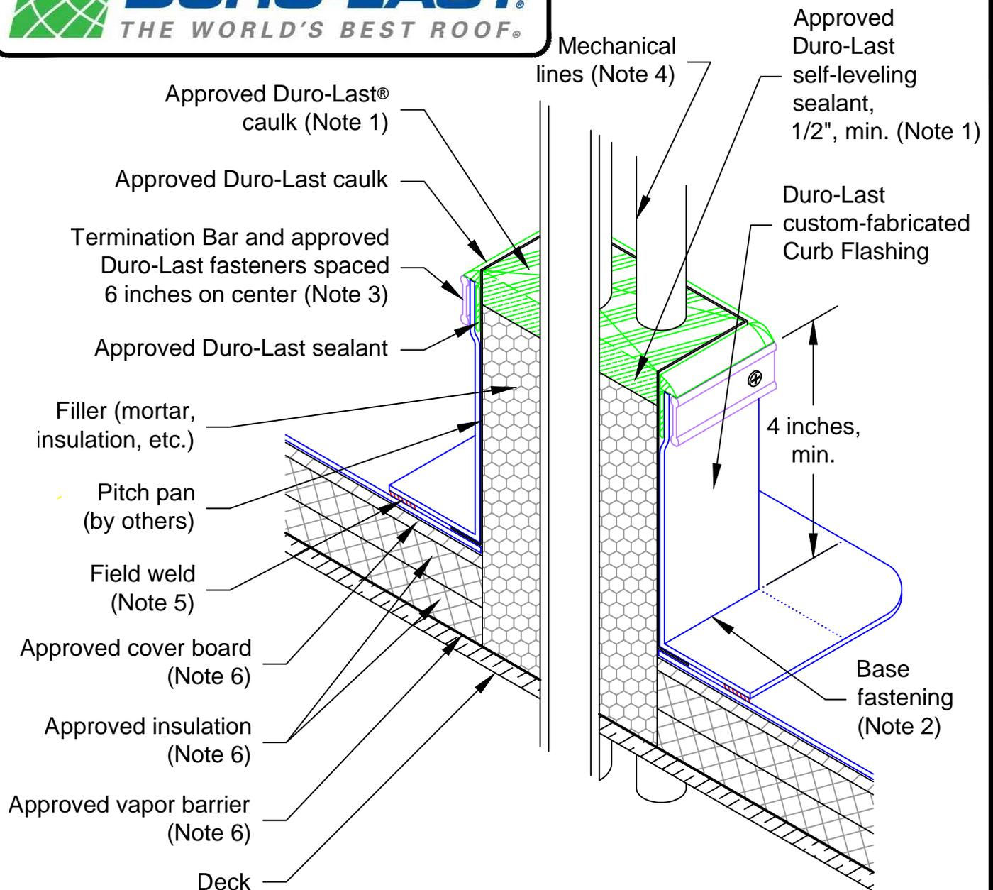
Note 1: Water must not be allowed to pond within pitch pan. Ensure that approved Duro-Last self-leveling sealant is level with top of curb. Cover with approved Duro-Last caulk to slope to outside of pitch pan.
