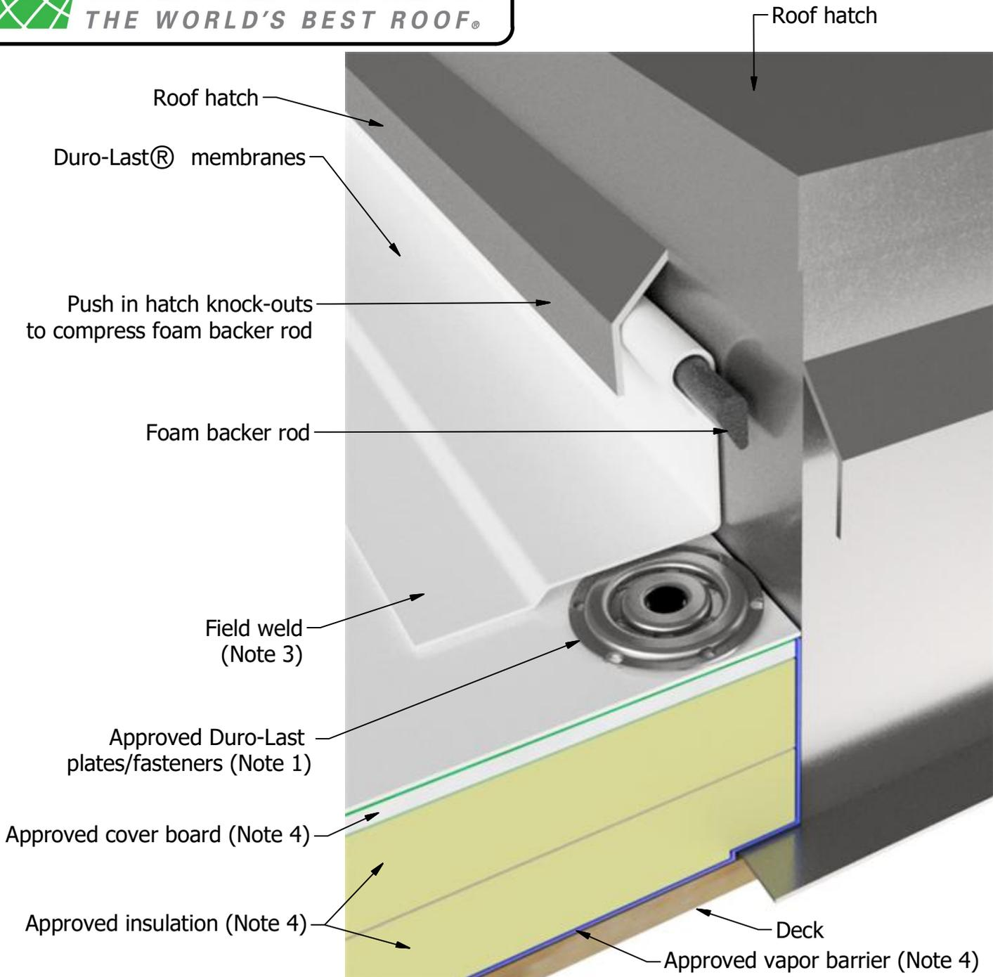
Note 1: Deck membrane shall be fastened around the perimeter of the roof access hatch as per the respective zone the roof access hatch is located within (field, perimeter, corner).
