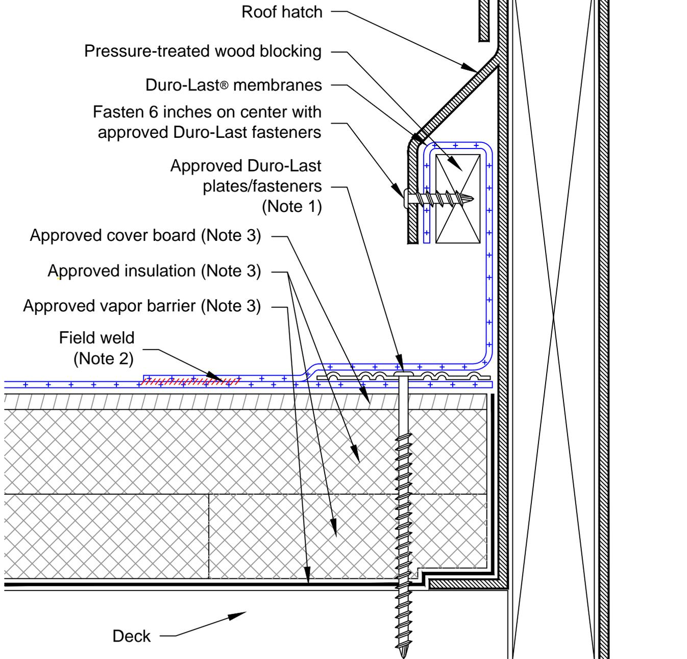
Note 1: Deck membrane shall be fastened around the perimeter of the roof access hatch as per the respective zone the roof access hatch is located within (field, perimeter, corner).
