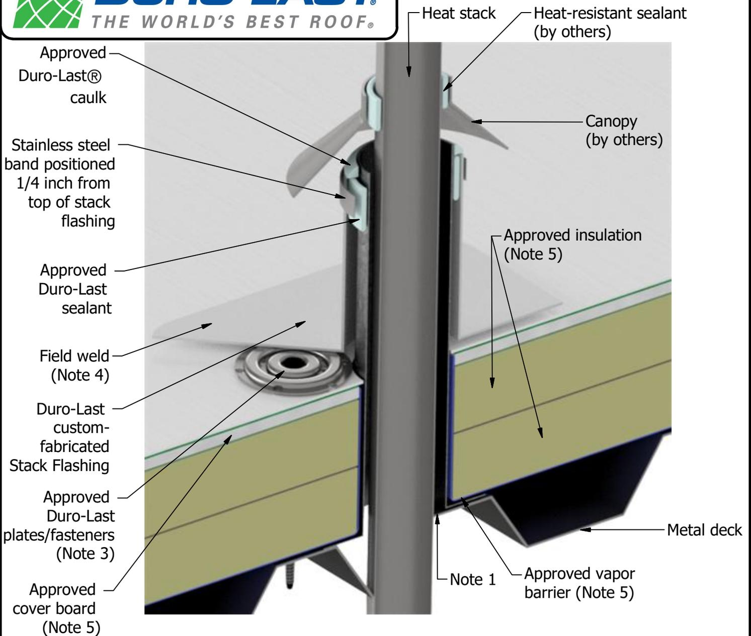
Note 1: This detail is required around heat stacks that exceed 120 degrees F, including all insulated chimney stacks. A minimum of 1-inch air space is required between the metal collar and heat stack. The canopy must be positioned to allow adequate air flow above the termination.
